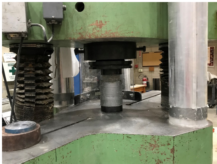
Figure 3-1. SATEC Machine for Cylinder Test
