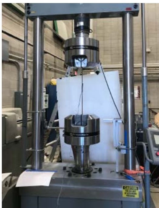
Figure 3-2. Steel Uniaxial Tensile Test Setup
