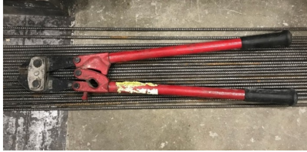
Figure 3-4. Bolt Cutter Used in Cutting NO.2 Bars
